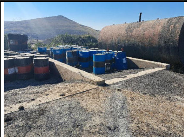
Bitumen products contained to a bunded area
