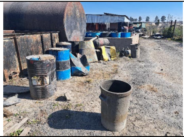
Drums to be moved to bunded areas with impermeable surfaces
