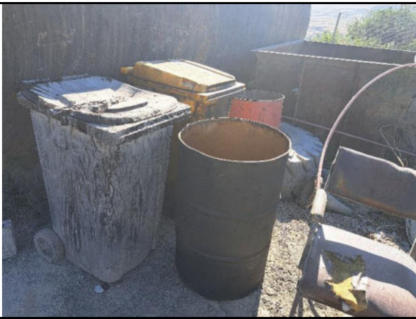
Drums to be moved to bunded areas with impermeable surfaces
