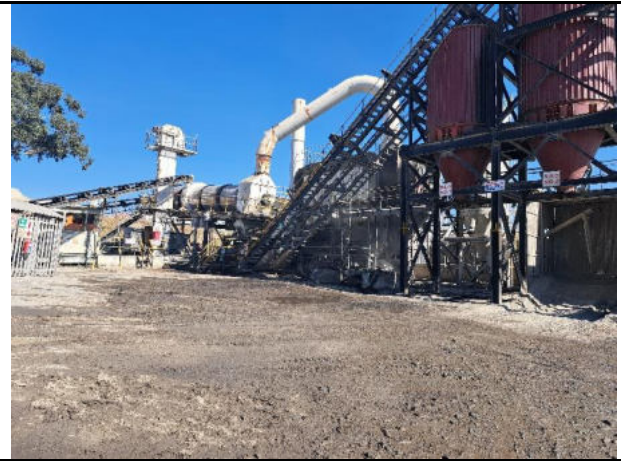
Old bitumen and contaminated soil contained to be reused in asphalt process
